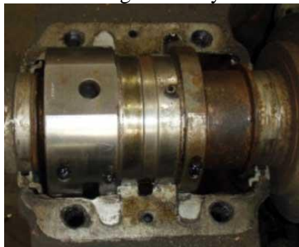
Failure of this bearing was caused by water ingress.
