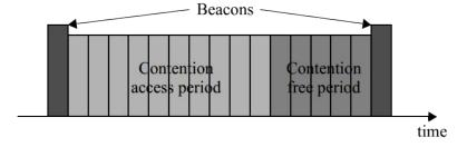
Figure 5-6—Structure of the active periods with GTSs
