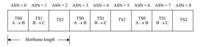
Figure 6-9—Example of a three time-slot slotframe
