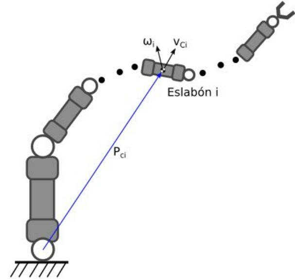
$$\mathbf{J}_{v_i} = \left[ \frac{\partial P_{C_i}}{\partial q_1}, \frac{\partial P_{C_i}}{\partial q_2}, \dots, \frac{\partial P_{C_i}}{\partial q_i}, 0, \dots, 0 \right]$$
