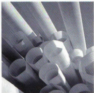
Ribbed plastic pipes stacked near a road construction site where they will be laid for drainage along the sides of a new section of motorway.
