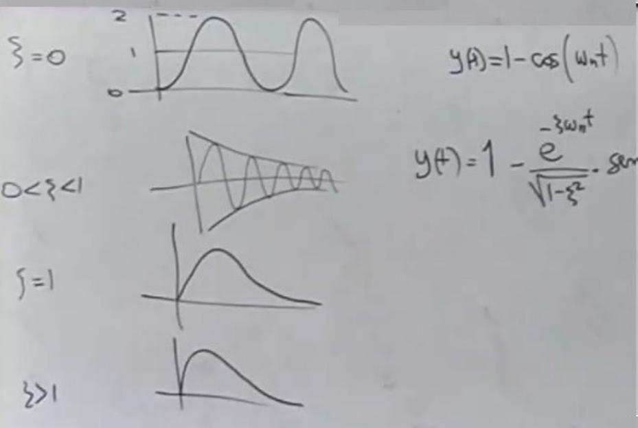
$$y(t) = 1 - \frac{e^{-\zeta \omega_n t}}{\sqrt{1-\zeta^2}} \sin\left(\underbrace{\omega_n \sqrt{1-\zeta^2}}_{\omega_d} t + \arctan\left[\underbrace{\frac{\sqrt{1-\zeta^2}}{\zeta}}_{\beta}\right]\right)$$
