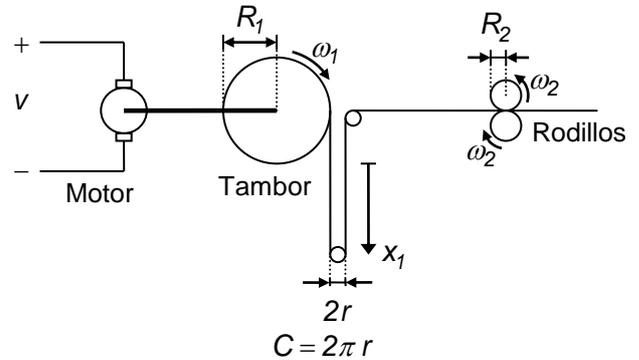
El motor cargado se modela mediante:  $\omega_1(s) = \left( \frac{a}{s+a} \right) \left( \frac{b}{s+b} \right) v(s) = \left( \frac{a}{s} \right) \left( \frac{b}{s} \right) \left( \frac{1}{1+\frac{a}{s}} \right) \left( \frac{1}{1+\frac{b}{s}} \right) v(s)$ .
