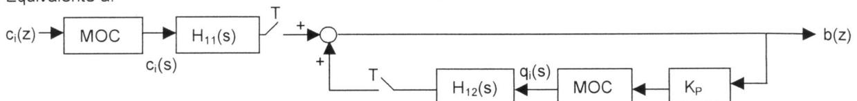
$$T_{LC}(z) = \frac{b(z)}{c_i(z)} = \frac{\bar{H}_{11}(z)}{1 - \bar{H}_{12}(z)K_P} \text{ donde:}$$
