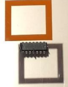
7474 TTL Flip-Flop, Texas Instruments, US, 1966 102716395
