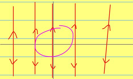
$$\begin{pmatrix} \dot{x}_1 \\ \dot{x}_2 \end{pmatrix} = \begin{pmatrix} 0 & 1 \\ 0 & 0 \end{pmatrix} \begin{pmatrix} x_1 \\ x_2 \end{pmatrix}$$
