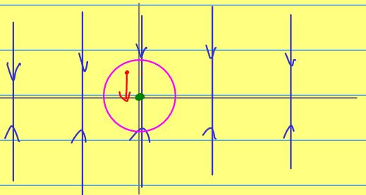
$$\begin{pmatrix} \dot{x}_1 \\ \dot{x}_2 \end{pmatrix} = \begin{pmatrix} 0 & -1 \\ 0 & 0 \end{pmatrix} \begin{pmatrix} x_1 \\ x_2 \end{pmatrix}$$
