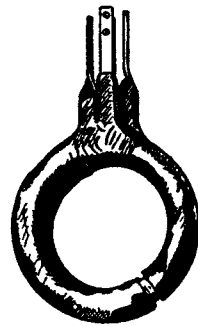
Primary Coil with Insulation ruptured by Hoop Tension.
