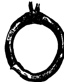
Primary Coil showing deformation of parts near Iron Core.
