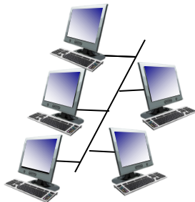
shared wire (e.g., cabled Ethernet)
