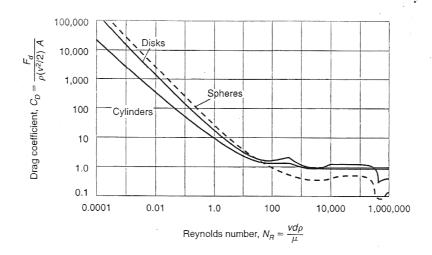
particle shape affects the value of the drag coefficient, for particles that are approximately spherical, the curve on Fig. 5–20 is approximated by the following equation (upper limit of  $N_R = 10^4$ ):
