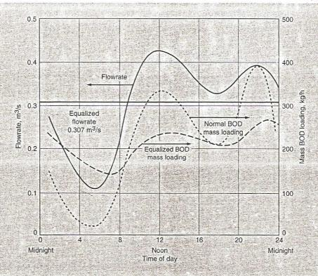
Comment Where in-line equalization basins are used, additional damping of the BOD mass loading rate can be obtained by increasing the volume of the basins. Although the flow to a treatment plant was equalized in this example, flow equalization would be used, more realistically, in locations with high infiltration/inflow or peak stormwater flows.
