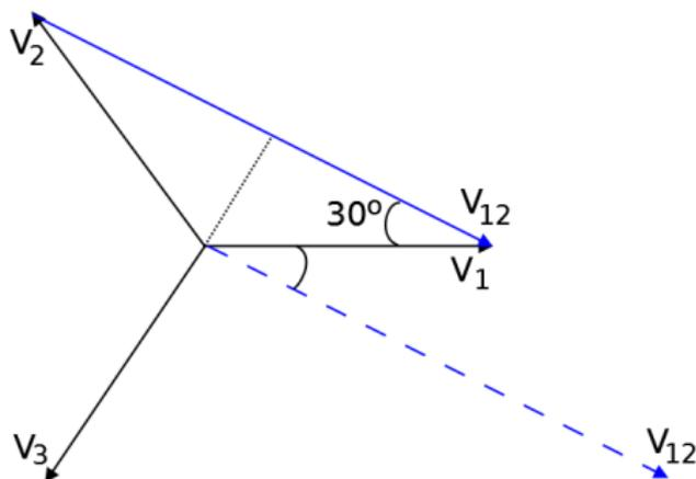
Tenemos que  $|V_{12}| = 2|V_1| \cos(\Phi) = 2|V_1| \cos(30^\circ) = 2|V_1| \frac{\sqrt{3}}{2} = \sqrt{3}|V_1|$  y  $\angle V_{12} = -30^\circ = -\frac{\pi}{6}$ .
