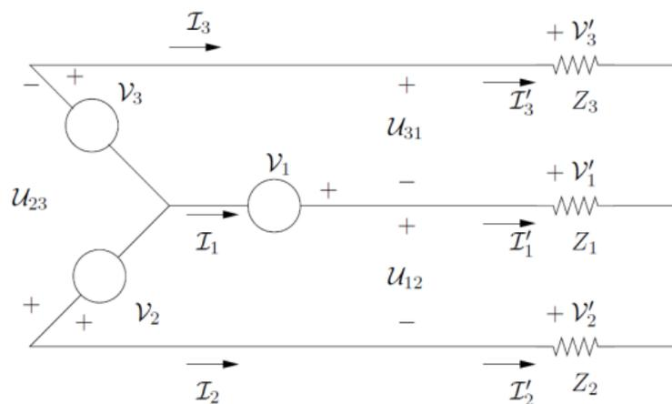
$$\begin{cases} I_1 = I'_1 \\ I_2 = I'_2 \\ I_3 = I'_3 \\ U_{12} = V'_1 - V'_2 \\ U_{23} = V'_2 - V'_3 \\ U_{31} = V'_3 - V'_1 \end{cases}$$
