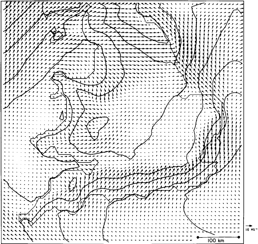
Fig. 13-5. The 50-m wind and sea-level pressure forecast for 1800 LST on June 14, 1973. The experiment includes orographic effects, the movement of a synoptic-scale anticyclone, and differential heating between land and water. The isopleth interval is 0.5 mb. One grid interval corresponds to 10 \text{ m s}^{-1} . (From Carpenter 1979.)
