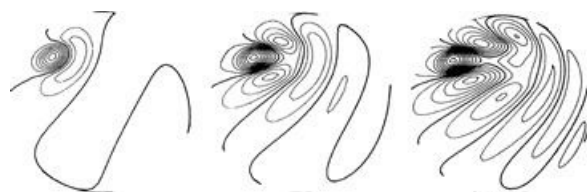
Figure 10.16 Vorticity pattern generated on a sphere when a constant angular velocity westerly flow impinges on a circular forcing centered at 30^\circ N and 45^\circ W of the central point. Left to right, the response at 2, 4, and 6 days after the forcing is switched on. Five contour intervals correspond to the maximum vorticity response that would occur in 1 day if there were no wave propagation. Heavy lines correspond to zero contours. The pattern is drawn on a projection in which the sphere is viewed from infinity.
