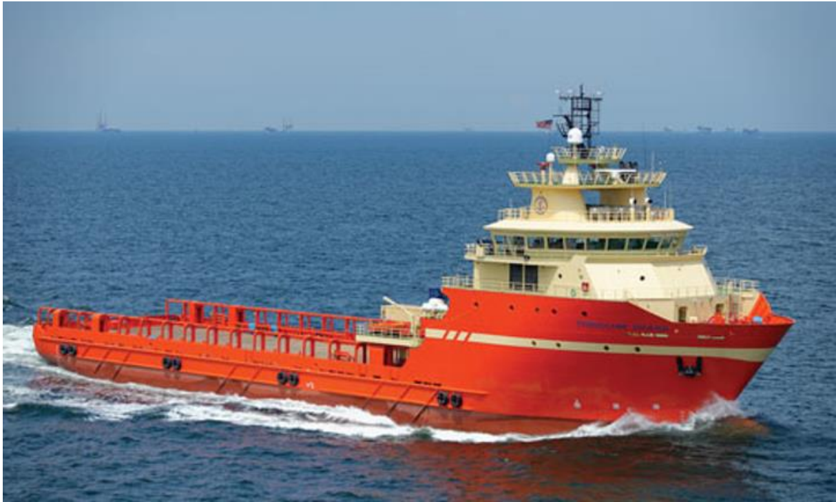
Fig. 11 - Buque de Suministro OSV (Offshore Supply Vessel)
