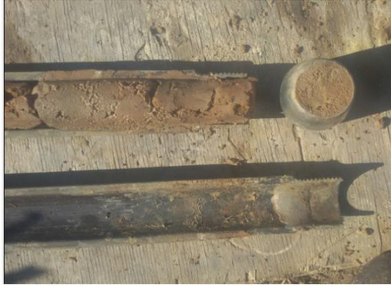
**ENSAYO S.P.T. a 8.8 m**
