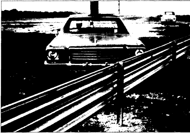
FIGURE 5.7 Weak Post Thrie-Beam Barrier
