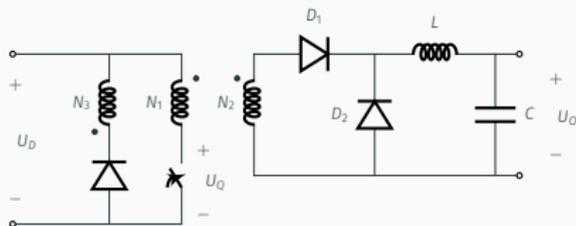
$$U_{Qmax} = U_{Dmax} + \frac{N_1}{N_3} U_{Dmax} = 152 \text{ V}$$
