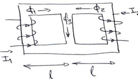
$$2) \text{ material lineal: } H = \frac{B}{\mu} = \frac{\Phi}{\mu S}$$
