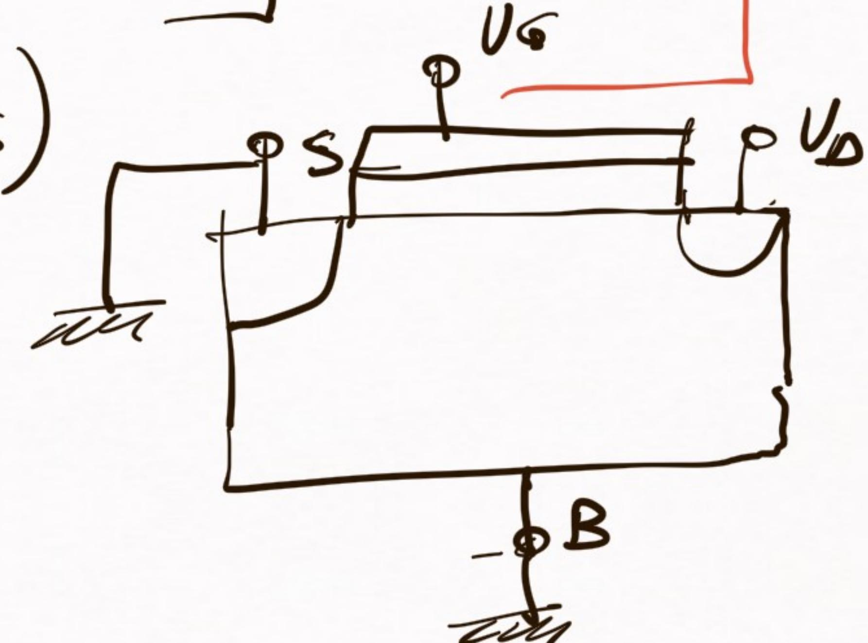
$$\Rightarrow I_D = \beta \left[ V_E - V_{TO} - \frac{(1+\delta)}{2} I_D \right] V_D \\ = \beta \left[ (V_E - V_{TO}) V_D - \frac{1+\delta}{2} I_D^2 \right]$$
