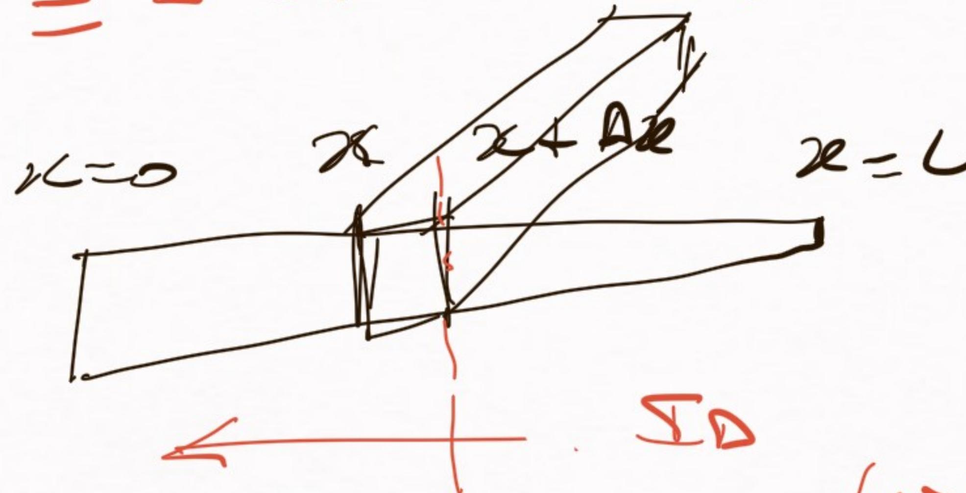
$$\Sigma D = \frac{\Delta Q}{\Delta f} = \frac{\Delta Q}{\Delta x} \cdot \frac{\Delta x}{\Delta t} = N_d \quad (\text{velocidad de los portadores})$$
