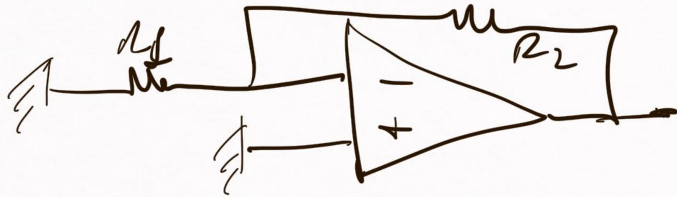
$$v_o = \left(1 + \frac{R_2}{R_1}\right) v_{offset}$$
