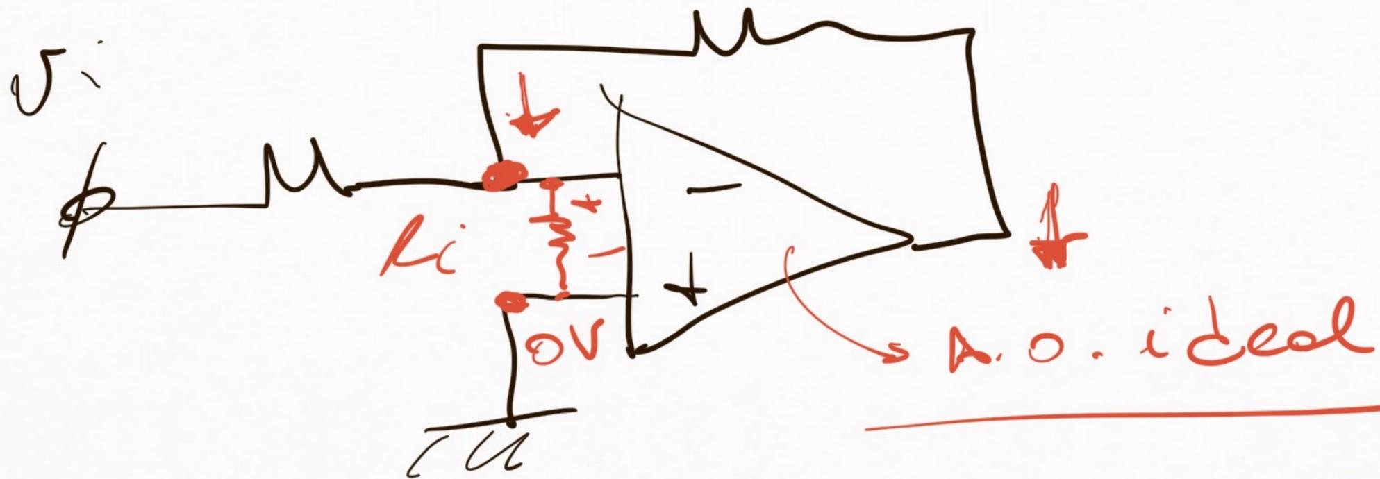
$$\underline{v_i \rightarrow 0} \rightarrow \left( \underline{v_o = -A \cdot v_i} \right) \Rightarrow \underline{v_o}$$
