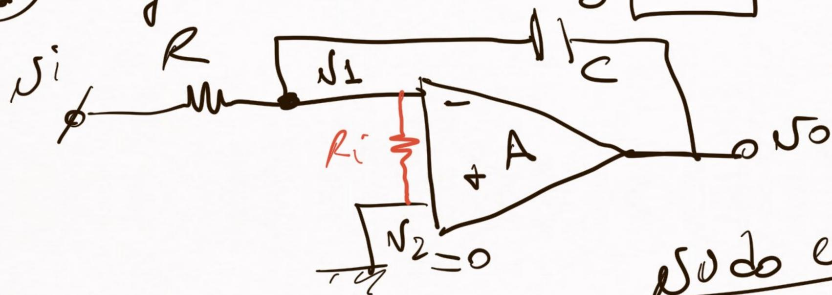
$$v_o = A(v_2 - v_1)$$
