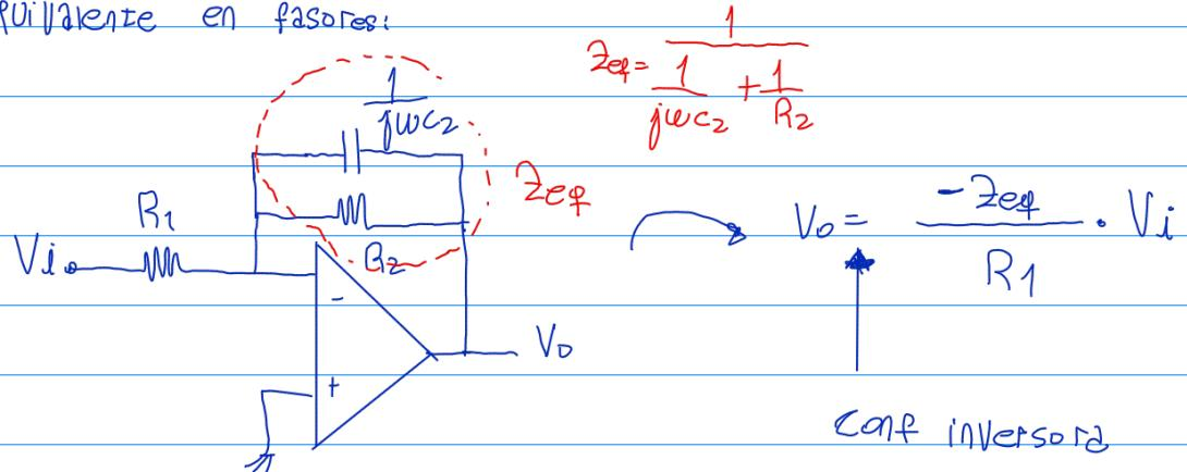
$$\frac{V_o(j\omega)}{V_i(j\omega)} = -\frac{R_2}{R_1} \cdot \left( \frac{1}{j\omega + \frac{1}{R_2 C_2}} \right) \cdot \frac{1}{R_2 C_2} = H(j\omega)$$
