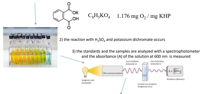
4) The calibration curve 'ABSORBANCE vs COD' is prepared with the standard solution (see point 1)
