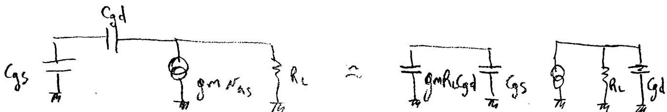
$$C_{gs} = \frac{2}{3} W \cdot L \cdot C_{ox} + C_{gs,ov} \cdot W = 0,33 \text{ pF}$$
