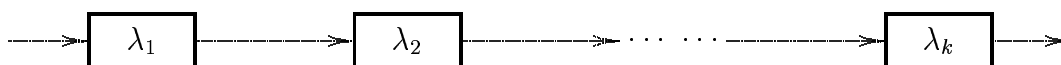
Figure 4.2: By combining k exponential distributions in series we get a steep distribution ( \varepsilon \leq 2 ). If all k distributions are identical ( \lambda_i = \lambda ), then we get an Erlang- k distribution.
