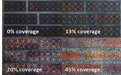
DSD PV: PV modules partly covered with a full color print (ECN).
