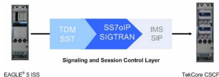
Figure 1. Transition from SS7 to IMS
