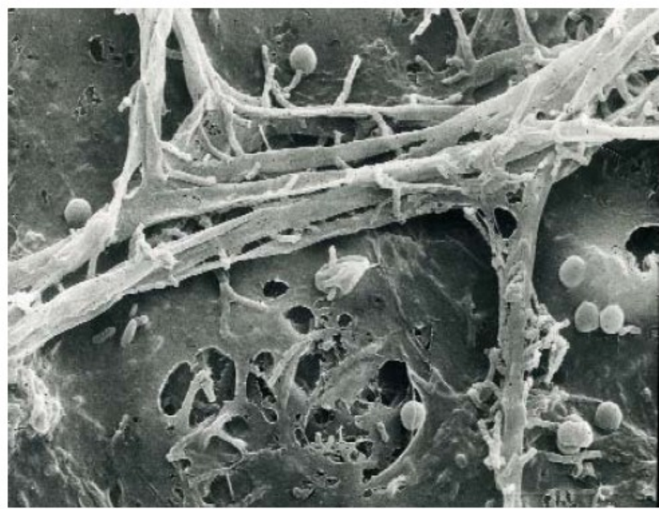
Figure 1. Biofilm on the surface of a water distribution system used in a dialysis unit. (Photographs courtesy of Luc Marchal and Jean Printz. Published with permission from Gambro Lundia AB, Lund, Sweden).
