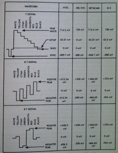
Figure 2.83 Analog component Y, B-Y, R-Y signal characteristics-100% color bars
