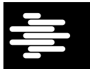
Figure 35.3 The weave technique stitches two fields into a frame. When applied to moving objects, it produces the "field tearing," "mouse's teeth," or "zipper" artifact.
