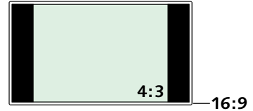
Figure 1.15 Pillarbox format (sometimes called sidebar ) fits narrow-aspect-ratio material to the height of a 16:9 display.
