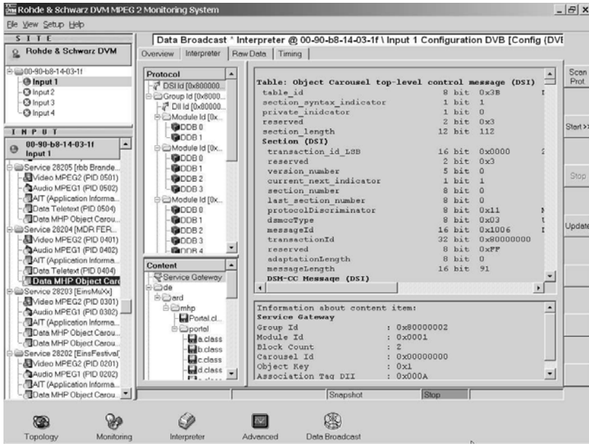
Fig. 27.6. MHP file structure of an object carousel as analyzed on an MPEG analyzer [DVM]
