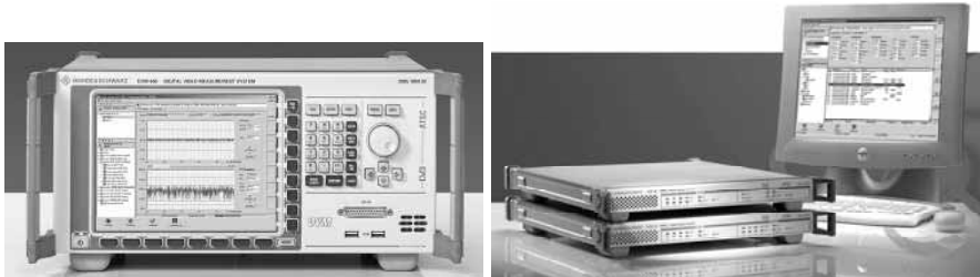
Fig. 11.11. MPEG-2 analyzer, Rohde&Schwarz, on the left: DVM400, on the right: DVM100
