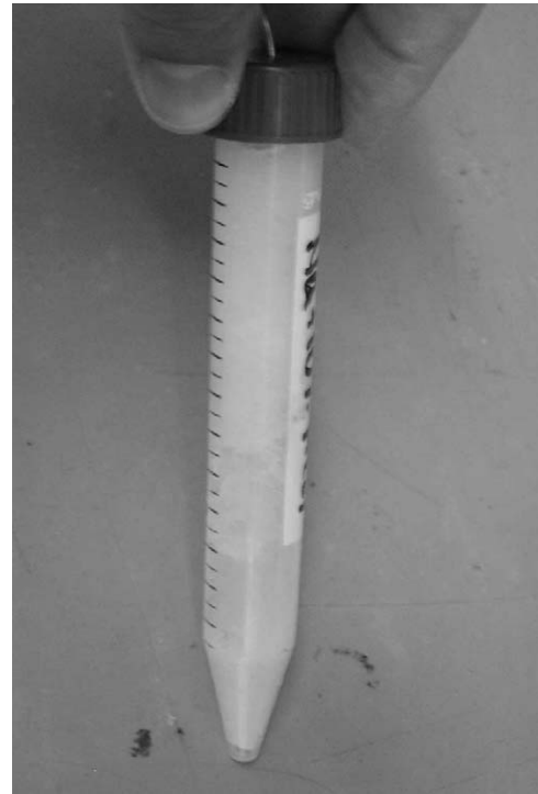
Fig. 9. Segregation of a salt hydrate [4].
