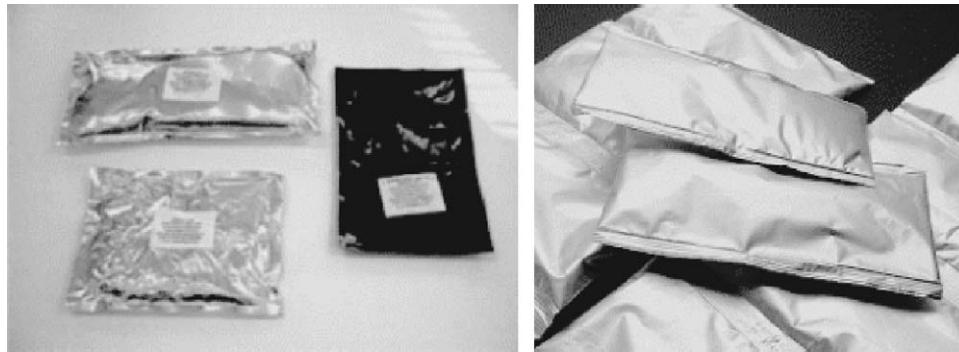
Fig. 17. Macro encapsulation in bags. Left – from Climator/Sweden; right – from Dörken/Germany [6].
