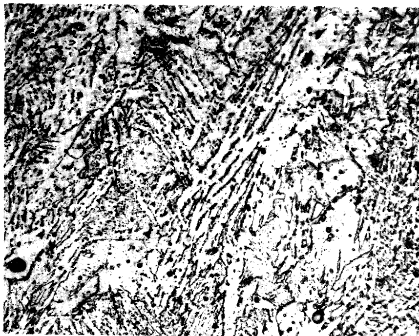
FIG. 46: WELD METAL, POSTHEATED WELD, E-6020 ELECTRODE, X500.
