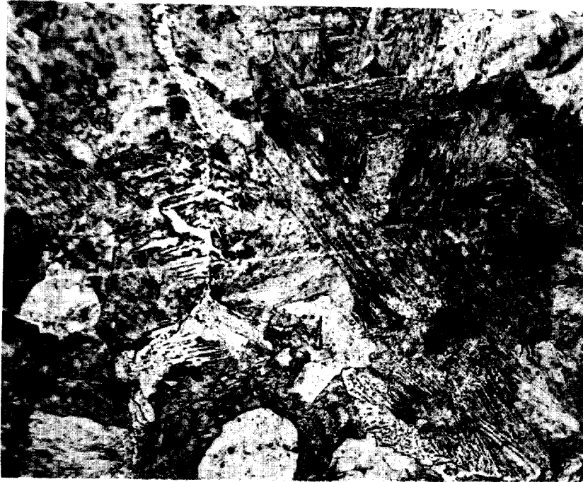
FIG. 47: HEAT AFFECTED ZONE, NON-POSTHEATED WELD, E-6010 ELECTRODE, X500.
