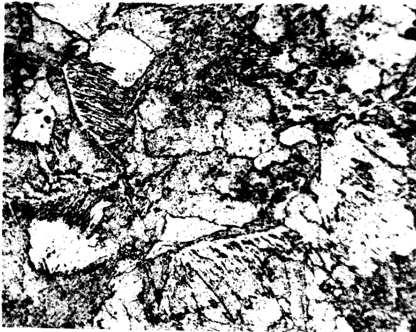
FIG. 48: HEAT AFFECTED ZONE, POSTHEATED WELD, E-6010 ELECTRODE, X500.
