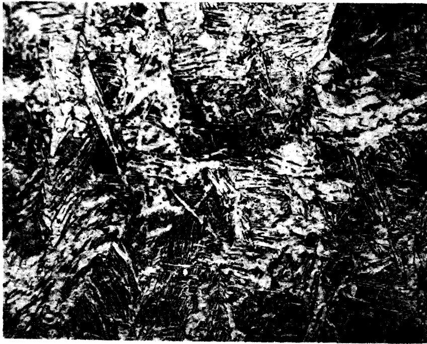
FIG. 43: WELD METAL, NON-POSTHEATED WELD, E-6010 ELECTRODE, X500.
