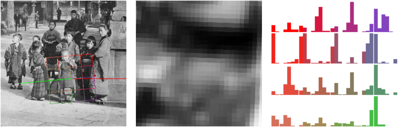
Figure 9: SIFT descriptor construction. No explicit re-sampling of the described normalized patch is performed. The normalized patch \mathcal{P}^{\text{descr}} is partitioned into a set of n_{\text{hist}} \times n_{\text{hist}} subpatches (default value n_{\text{hist}} = 4 ). Each sample (m, n) inside \mathcal{P}^{\text{descr}} , located at (m\delta^o, n\delta^o) , contributes by an amount that is a function of their normalized coordinates (\hat{x}_{m,n}, \hat{y}_{m,n}) (see (24)). Each sub-patch \mathcal{P}_{(i,j)}^{\text{descr}} is centered at (\hat{x}_i, \hat{y}_j) .
