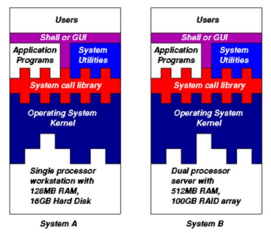
Fig. 1.1: General operating system architecture
