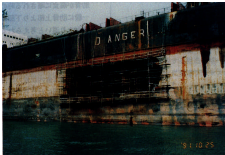
Photograph 2 Missing side shell structure (See Examples 4 and 5)
