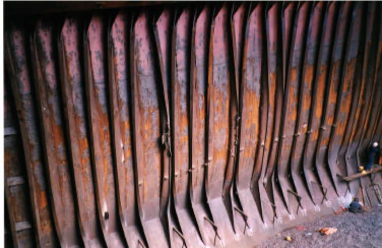
Photograph 1 Collapsed side shell frames (See Example 4)
