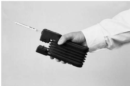
Figure 3.6.3 Draeger bellows pump and tube. (Courtesy Draeger Ltd)
