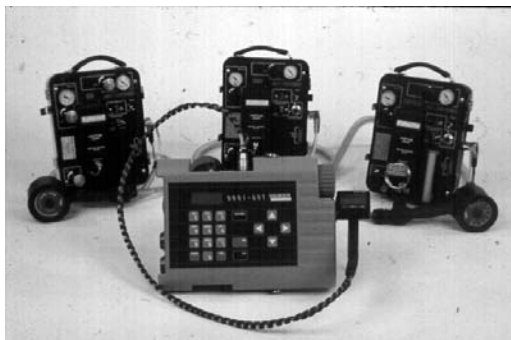
Figure 3.3.9 Organic vapour analyser. (Courtesy Quantitech Ltd)
