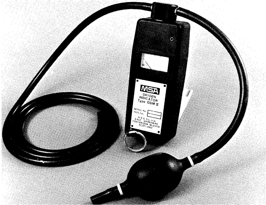
Figure 3.3.11 Portable oxygen analyser. (Courtesy M.S.A. Ltd)
