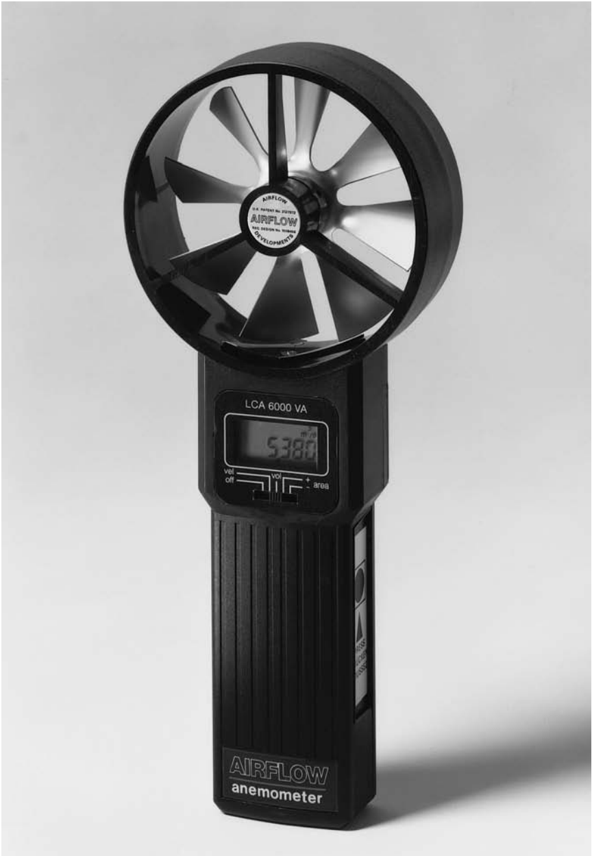
Figure 3.6.7 Vane anemometer. (Courtesy Air Flow Developments Ltd)
