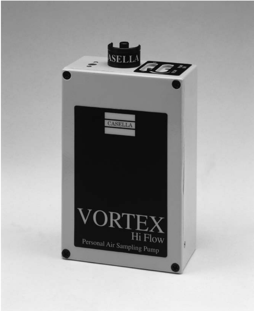
Figure 3.6.2 Personal dust sampling pump. (Courtesy Casella Ltd)
