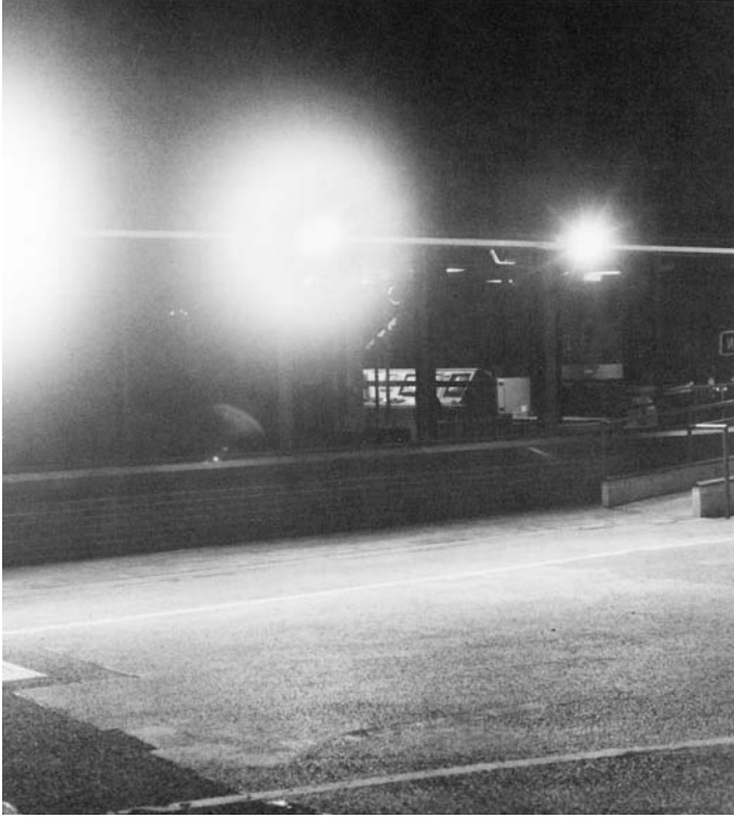
Figure 3.9.15 Disability glare from a light fitting (Courtesy The Stationery Office)
