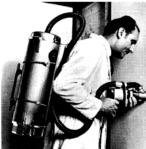
Figure 3.6.4 High velocity low volume extractor. (Courtesy BVC Ltd)
