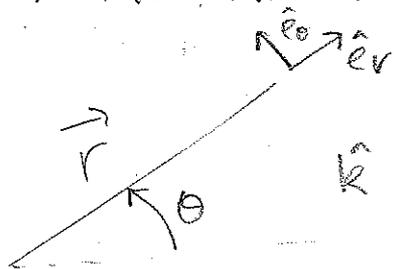
$$\left. \begin{aligned} \vec{r} &= r \hat{e}_r \\ \vec{v} &= \dot{r} \hat{e}_r + r \dot{\theta} \hat{e}_\theta \end{aligned} \right\} \vec{L} = \underbrace{m r^2 \dot{\theta}}_{l \text{ (cte)}} \hat{k}$$
