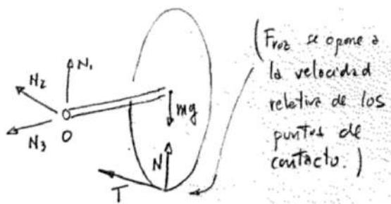
$$-\frac{ma^2}{2} \dot{\gamma} = +Ta ; \quad \frac{5ma^2}{4} \ddot{\phi} = +Ta ; \quad -\frac{ma^2}{2} \dot{\gamma} \dot{\phi} = (mg - N)\dot{\phi}$$
