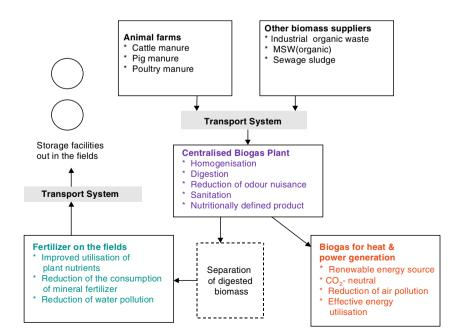
Fig. 2. The main streams of the integrated concept of centralized co-digestion plant (Holm-Nielsen and Al Seadi, 2004).
