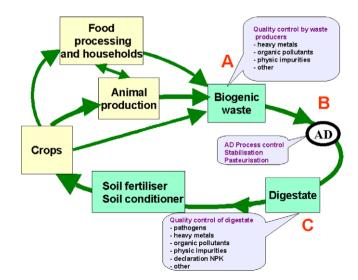
**Fig. 3.** Schematic representation of the closed cycle of anaerobic digestion of biogenic waste and the three main steps (A, B and C) of the quality management process (Al Seadi, 2002).
