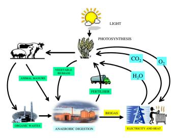
Fig. 1. Schematic representation of the sustainable cycle of anaerobic co-digestion of animal manure and organic wastes (Al Seadi, 2002).
