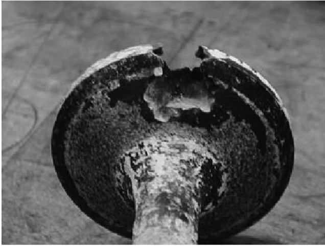
FIG. 12.1. Damage caused by hydrogen sulfide. Source: Applied Filter Technology. Reprinted with permission.
