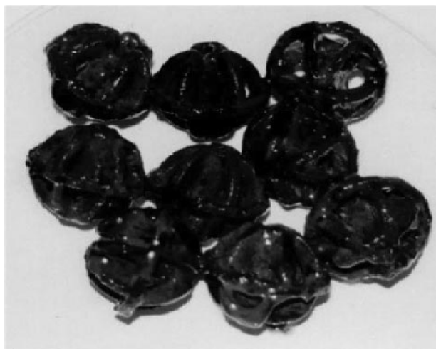
FIG. 5.6. Biofilm growth on support media.
