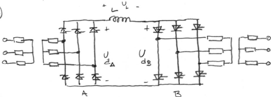
$$b) \langle I_T \rangle_{\text{tiristor}} = 1000 \text{ A} \Rightarrow I_d = 3 \langle I_T \rangle = 3000 \text{ A}$$
