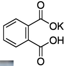
$$\text{C}_8\text{H}_5\text{KO}_4 \quad 1.176 \text{ mg O}_2 / \text{mg KHP}$$
