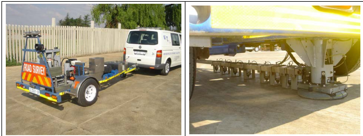
Figure 7. Falling Weight Deflectometer (FWD)
