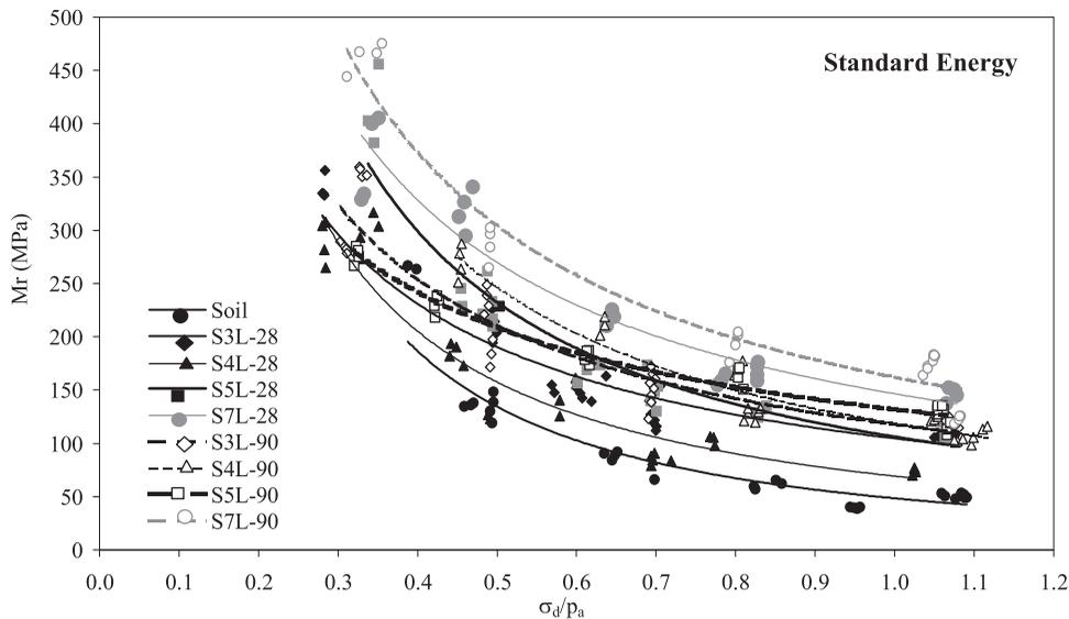
Figure 3. Resilient modulus of soil and soil treated with different lime contents and times compacted at standard energy as function of normalised deviator stress.
