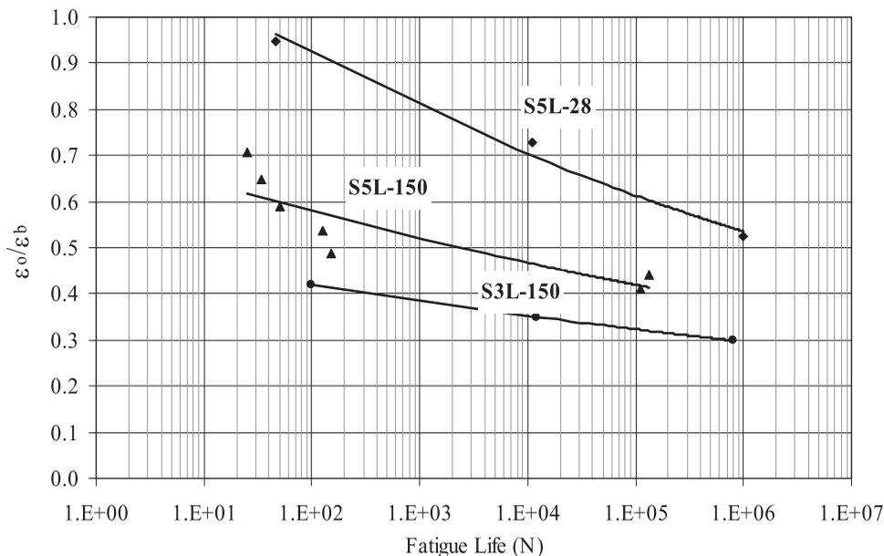
Figure 8. Fatigue life of soil modified with lime as function of the initial tensile strain-tensile strain at break ratio.
