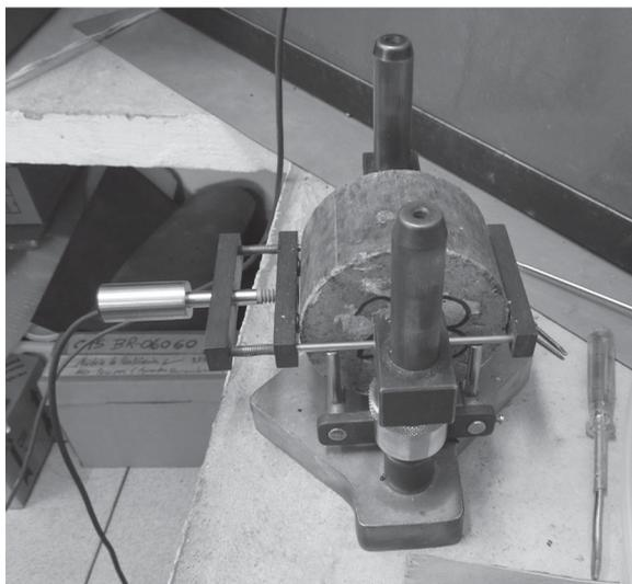
Figure 1. Strain measurement device used in fatigue life tests.
