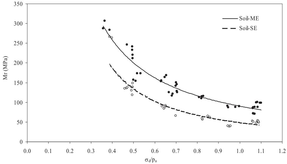
Figure 2. Resilient modulus of soil compacted at standard and modified efforts as function of normalised deviator stress.
