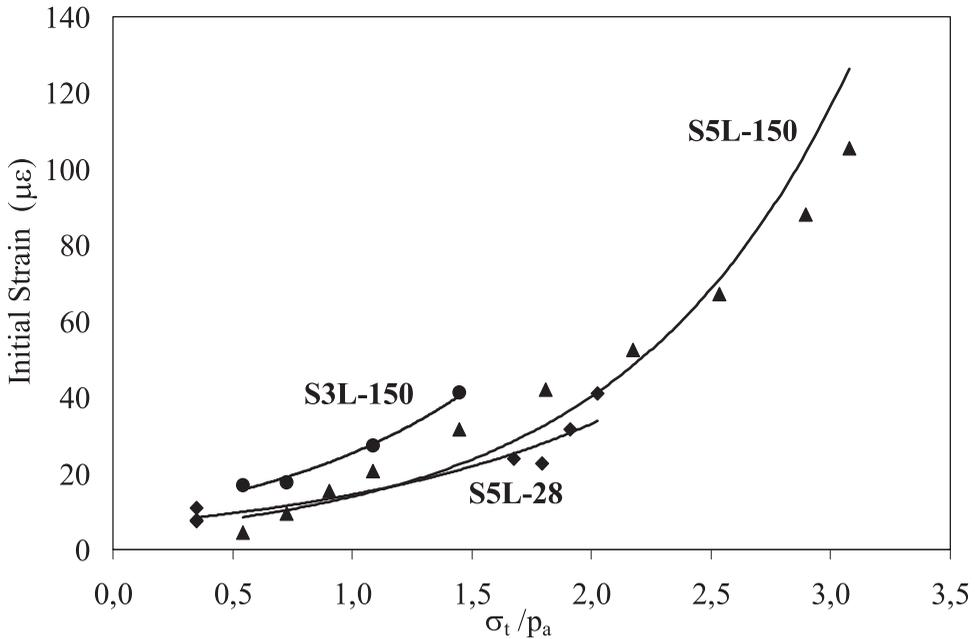
Figure 9. Initial tensile strain as function of the normalised tensile stress applied in fatigue life tests.
