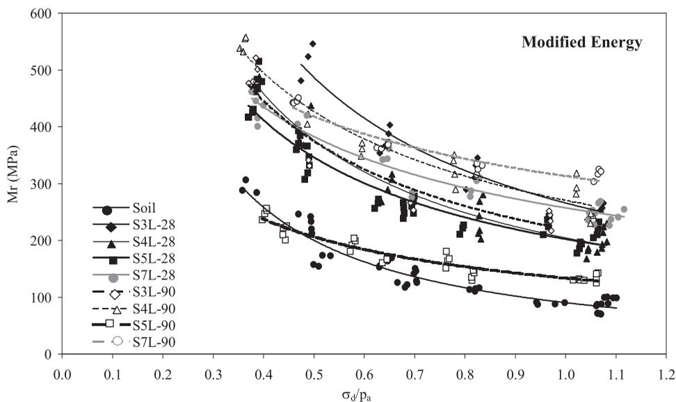
Figure 4. Resilient modulus of soil and soil treated with different lime contents and times compacted at modified energy as function of normalised deviator stress.
