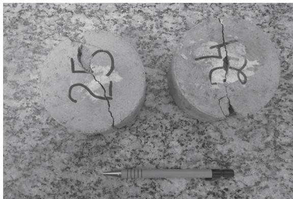
Figure 6. Break failure observed in fatigue life tests of clayey silt modified with lime.
