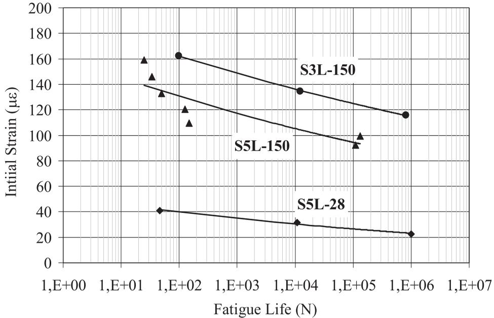
Figure 7. Fatigue life of soil modified with lime as function of the initial tensile strain.
