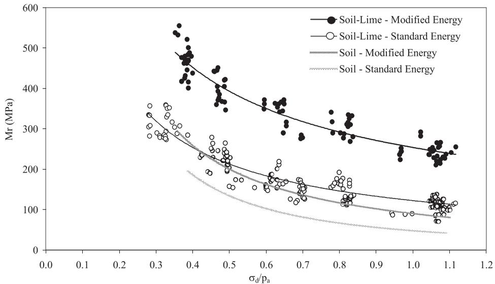
Figure 5. Resilient modulus of soil and soil modified with lime as function of normalised deviator stress contents and compaction energy.
