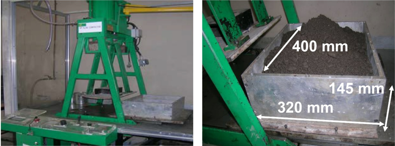
Figure 8.8: Compaction of test slabs from which test beams are sawn
