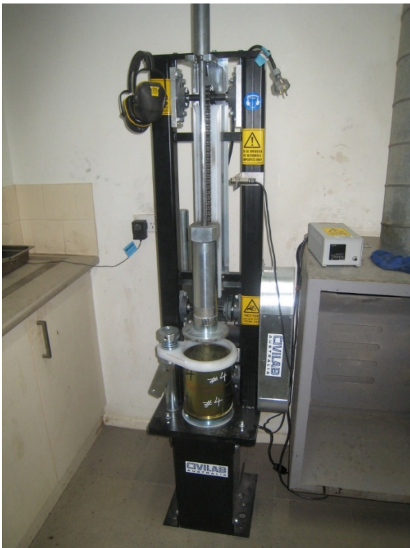
Figure 5.7: Large-scale Marshall mould and drop hammer
